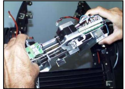
Fig. 21 Insert module at an angle
