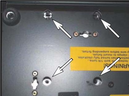
**Fig. 103 Ballast bracket screws**
