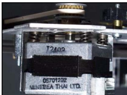
**Fig. 79** Flag motor suspension
