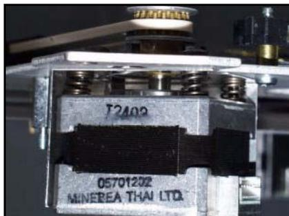
**Fig. 79** Flag motor suspension
