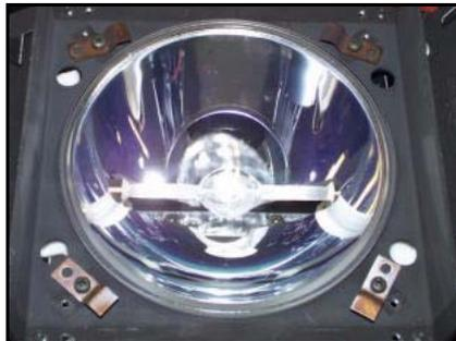
Fig. 44 Turn clips to free reflector
