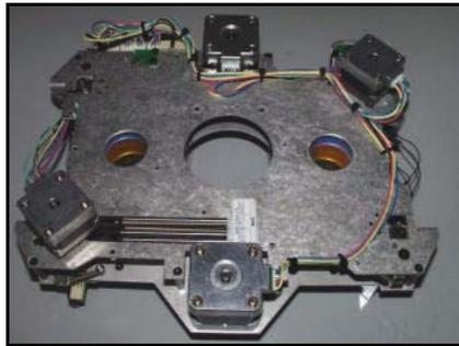
Fig. 59 Dimmer motor orientation
