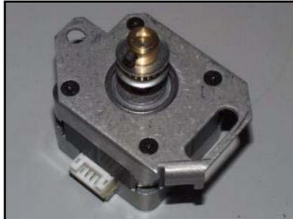
Fig. 27 Motor and bracket
