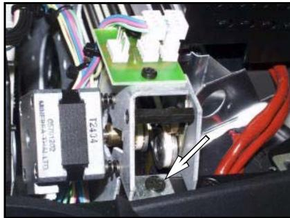
Fig. 20 1 of 4 CMYC module screws
