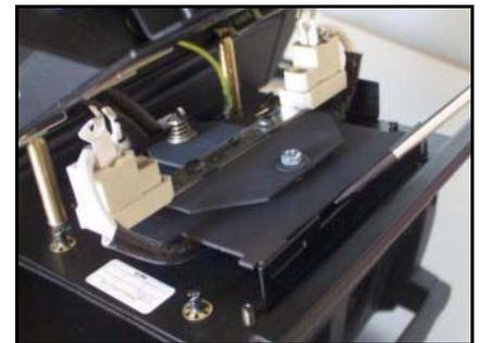
Fig. 46 Pry out the adjustment plate
