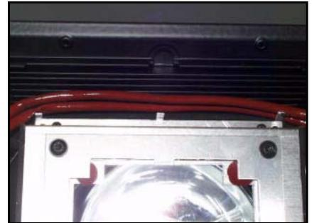
Fig. 39 Move wires out of way
