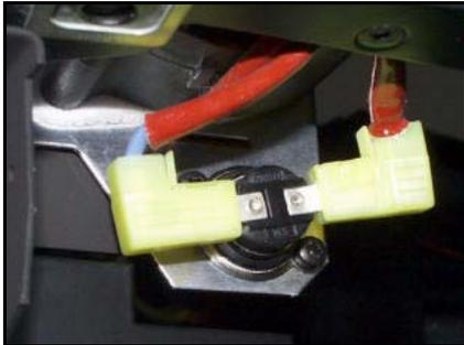
Fig. 36 Thermo-switch connections
