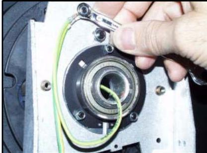
**Fig. 82** Disconnect ground wires
