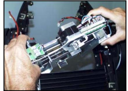
Fig. 21 Insert module at an angle
