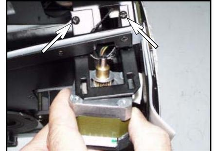
Fig. 15 Loosen bracket to remove motor
