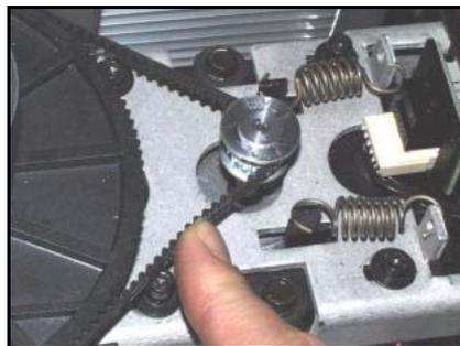
**Fig. 98 Check belt tension**
