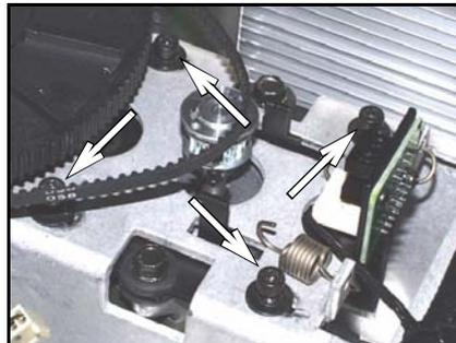
**Fig. 97 Motor bracket screws**
