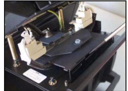
Fig. 46 Pry out the adjustment plate
