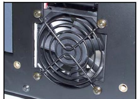
Fig. 109 Fan grill installation
