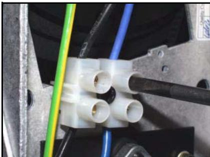
**Fig. 81** Disconnect lamp wires
