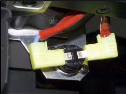
Fig. 36 Thermo-switch connections
