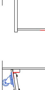
General method for lift units, Modify as needed, NOTE: Hinges NEVER bear the unit weight,
