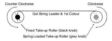
To apply tension to the gel string being loaded, the following procedure should be followed:
