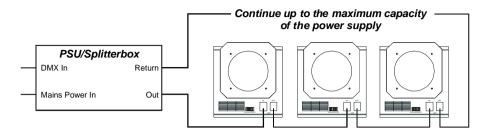
**Note:** Total cable length per circuit must not exceed 60m / 200' on the PS08 PSU / Splitterbox and 105m / 350' on the PS18/2 PSU / Splitterbox.
