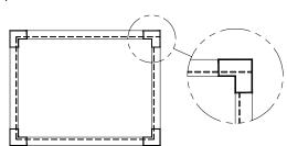
When mounting your DataTrack with data bus, please ensure that no loops within the data line are created. Failure to do so may result in unreliable data transmission.
