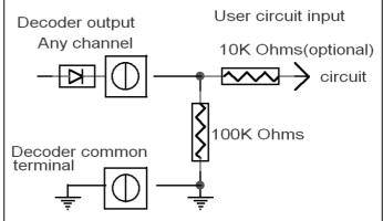
**Misc.** Good solid connections are a must. The micro screw terminals provide good connections. However the screws can be stripped by over tightening.
