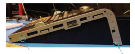
2) Remove 2 screws holding side cover, and remove cove. Repeat for opposite side.
