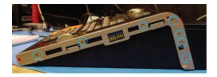
3) Remove 7 side screw indicated in blue. Leaving the 3 screws marked in red. Repeat for opposite side.
