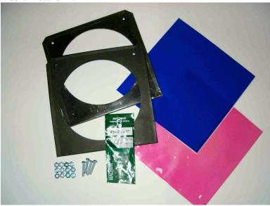
As Picture#1 shows, the only parts needed are two appropriately sized color frames, (4) #10-24 x 1" Round-Head Machine Screws, and (12) #10-24 hex nuts. The picture shows 7.5" x 7.5" color frames, but the color extender can be fabricated equally effectively from 6.25" or 10" frames.
