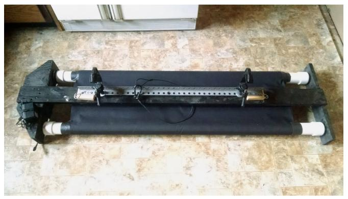
The machine is just over 5' long and 18" wide. Mounting is with the two standard c-clamps to 1.5" steel pipe. The safety cable should go around the wood backbone. A wall-wart style power supply is included and should be provided with switched power only (a D20 configured to switched mode is acceptable).
