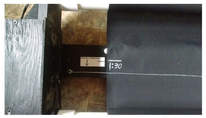
The fabric is marked in 10s increments from 0 to 1:30 and the arrow indicates the direction the motor moves the fabric. Since it moves at a constant rate, how densely the petals are loaded will determine how many fall at once. There's a little extra fabric after 1:30 and no immediate harm will come from running all the way to the end. However, it's best to shut it off before the end to avoid straining the motor.
