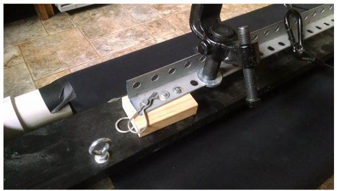
A pin is provided at each end to remove the machine from the hanging bracket. This makes it easier to flip over and fill. Also note the gaff tape holding the fabric to the PVC. This prevents it from unrolling in transport.
