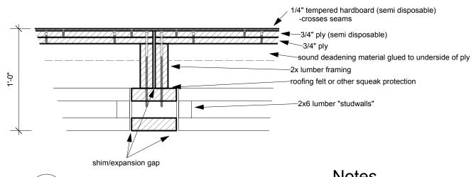
stage system section detail 2 Scale: 1 1/2" = 1'-0"
