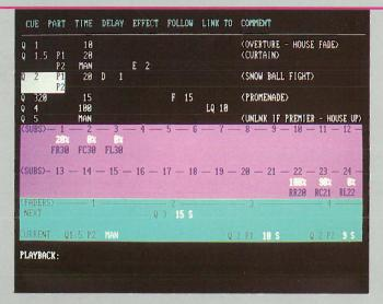
The **Playback** function display is a color, three-part screen which lays out the status of the current fader, cuesheet and submaster activity. The easy-to-read information is laid out to be clear and precise. As this information appears on your left monitor it provides you with instant reference to immediate and pending cues, so you are always in control and on top of your show.
