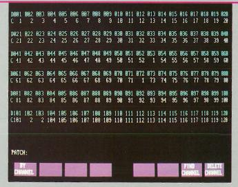
The Patch display permits you to speedily patch up to 800 dimmers to the Prestige 3000's 400 powerful control channels. Once you've set up, this graphic can show you your patch list in either dimmer or channel order, at your preference. Patch can also instantly search for and locate any channel or dimmer you specify. You can find, check and correct your patches quicker than ever.
