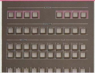
The Screen, Record, and Cue key pads are your fingertip controls for the flexibility of the Prestige 3000. The eight Screen Keys are soft keys whose functions are unique and tailored to each of the ten displays. Each of these independent controls is clearly labeled at the bottom of the selected display. Soft keys save clutter on the board since only the keys you need for the work you are doing are present. You'll work faster and more accurately.
