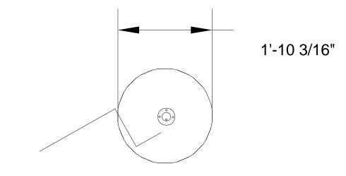
2" pipe flange mounted at center of 3/4" plywood "hub"
