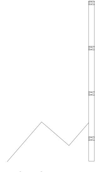
1"x3" with 2" STRAIGHT casters Placed at radii of arc peices. Build X's 16
